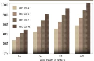
The throughput data indicated takes into account complete production runs for various wire lengths & for each model
